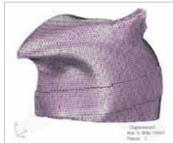
Mesh generated in Patran using the Marc Hex Mesher
